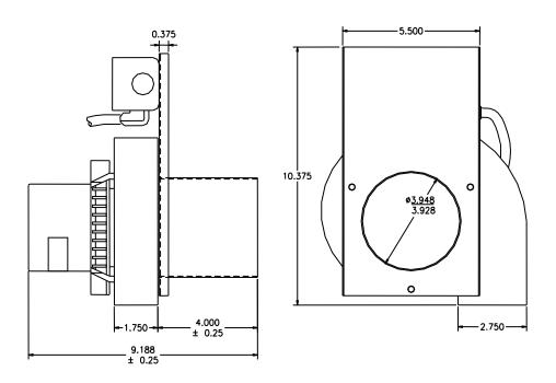
**NOTE** - Motor substitutions can occur, always refer to the motor manufacturer nameplate for electrical information and wiring instructions. Housings and inlets for 0101 vacuum exhauster made with stainless steel are also available – the last two-digit designation will be SS.
