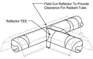
Use Sheet Metal Screws To Secure
