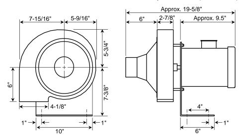
NOTE - Motor substitutions can occur, always refer to the motor manufacturer nameplate for electrical information and wiring instructions. Three phase and alternate voltage motors are available as a special order. Housings and inlets made with stainless steel are also available – the last two-digit designation will be SS.
