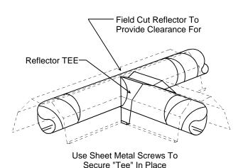
For "X" fittings (PN 0404.AS.X) use the same technique shown, cutting and another relief hole on the opposite side of the reflector and installing a second reflector tee.
