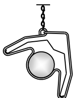
40° Mounting With “Combination” Hanger
